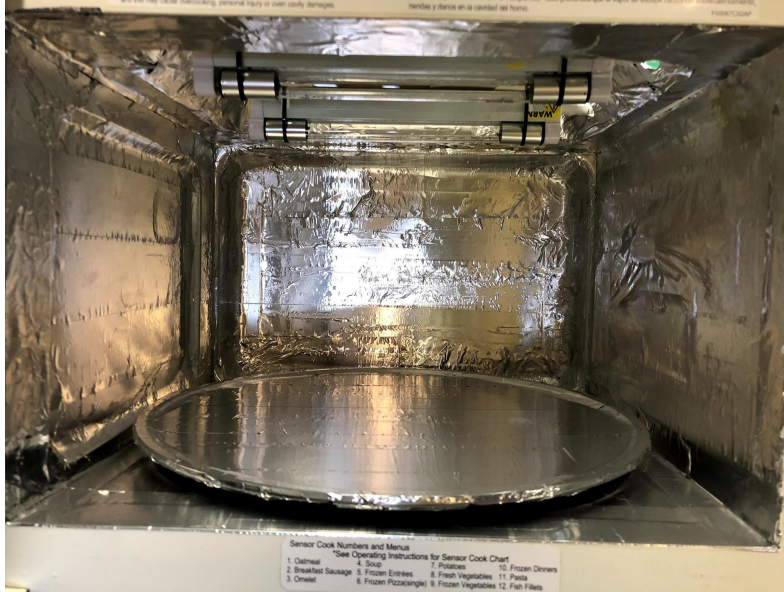
Figure 21: UV-C Lamps and Aluminium Tape Interior
