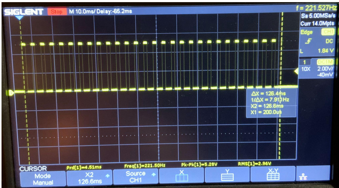
Figure 4: Incoming PWM sent by Microwave's MCU
