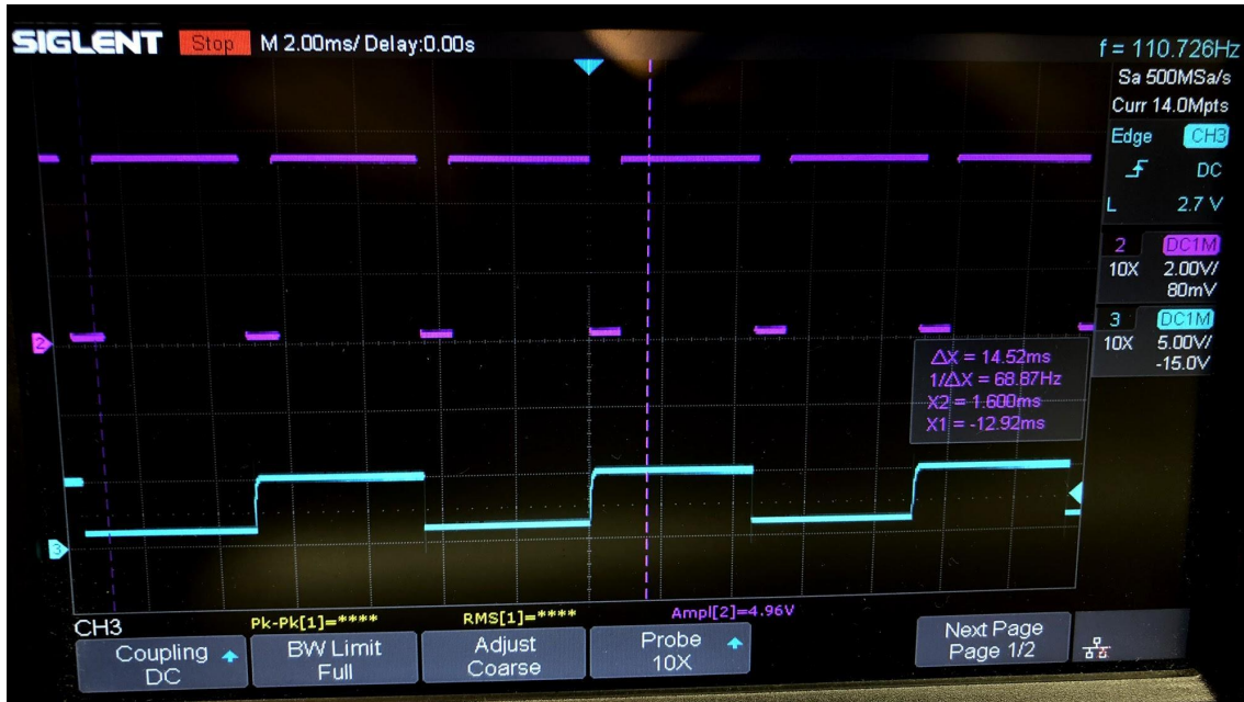
Figure 17: Input Pin (PWM) in Magenta and Output Pin (OSC) in Cyan
