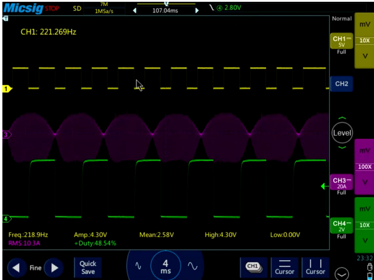
Figure 5: PWM and OSC signal (Credit to TomTechTod Youtube Channel)
